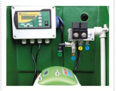
The air lines are properly connected when the correct color of the wire is leftplugged into the, correct connector:
