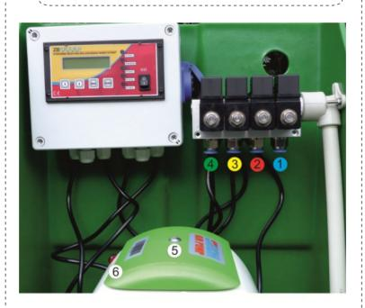
The air lines are properly connected when the correct color of the wire is leftplugged into the correct connector:
